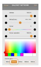
Maximum current that can be supplied by the device for each single output: 200mA
